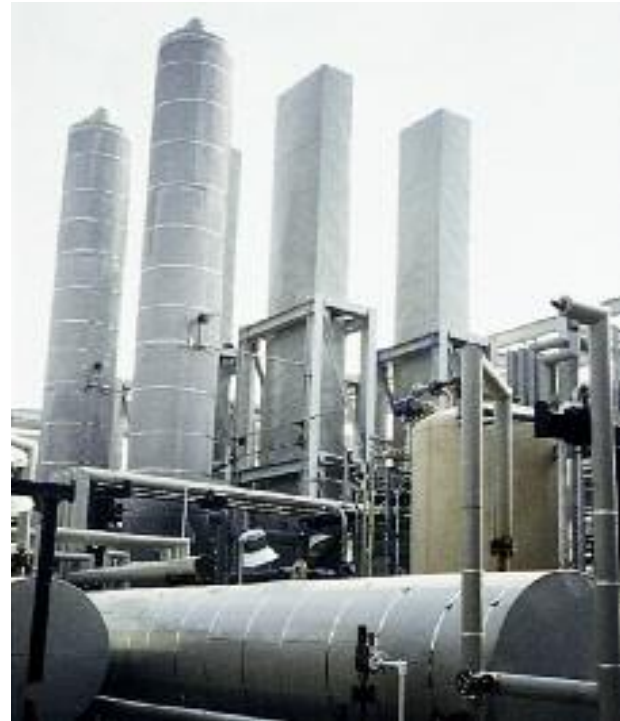
The Zimpro® wet oxidation system is used primarily for spent caustic waste treatment, but can be used successfully in other applications.
